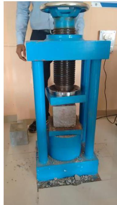
Fig – 3: Testing of concrete cubes
