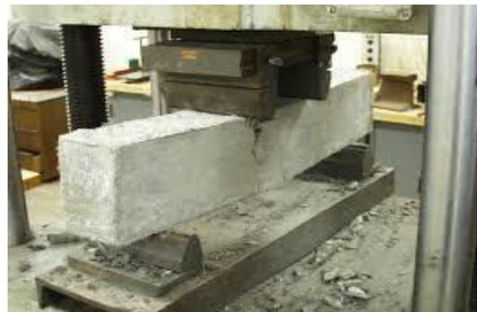
Fig – 4: Testing of concrete beams
